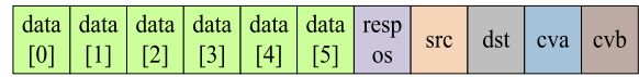
Fig. 7. Register communication protocol: The width of the whole packet is 256 bits. The front is 6 data locations, which occupies 192 bits. “Respos” occupies 16 bits and stores the offset of the packet in the CPE receiving buffer. “Src” records the data sender with 8 bits. The “dst” uses an 8-bit recording data receiver. “Cva” records 16 bits of valid data. “Cvb” is empty, which occupying 16 bits.
