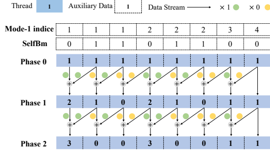
Figure 3: The illustration of inter-warp reduction for ALS.
